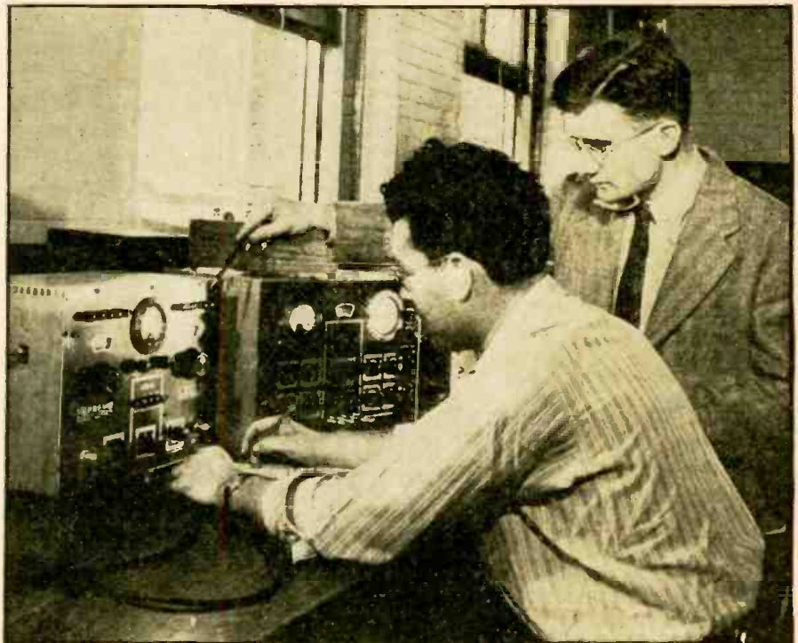
One of the several hundred Signal Corps enlisted reserves receiving special radio studies at this Midwest school. He is working with Instructor J. C. Abener. The two pieces of apparatus with which they are working are a signal generator and a vedolyzer. (Above)
